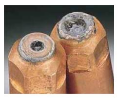
After the same number of starts, the Hypertherm electrode on the left shows a well-centered pit and is about half used. Due to poor manufacturing, the non-Hypertherm part on the right has eroded past the hafnium insert and must be replaced prematurely.
